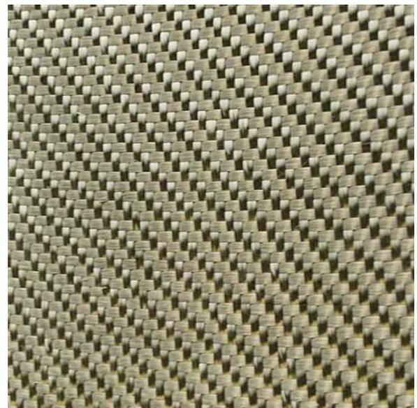
Basalt fibers have higher strength and elastic modulus than conventional E glass getting close to special high strength S glass and carbon fibers. So they offer for car makers an opportunity for significant cost reduction of SMC/BMC parts while keeping high strength and stiffness. The dielectric properties of basalt fibers are equal to ones of glass fibers. And switch from glass to basalt does not change radar transparency.
