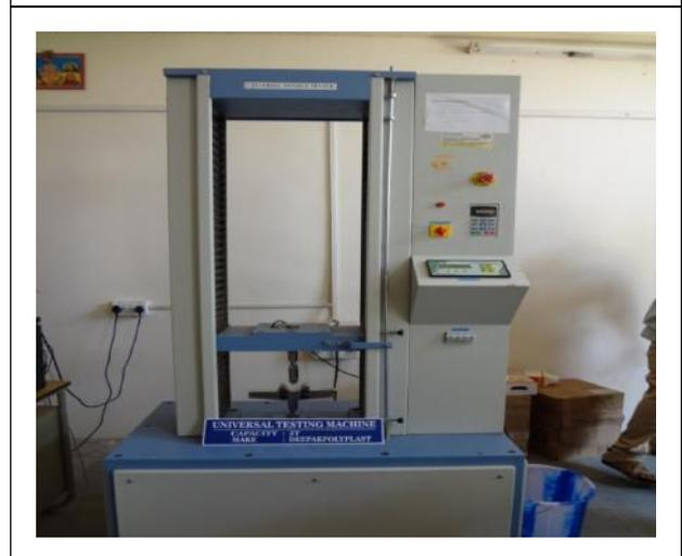
specimens are supported as a simple beam, with the compressive load applied at midpoint, and maximum fiber stress and strain calculated. The three point bending flexural test measures bend or fracture strength, yield strength, modulus of elasticity in bending, flexural stress, flexural strain, and flexural stress strain materials response. Flexural strength represents the highest stress experienced within the material at its moment of rupture.
