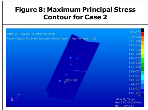
in case 1 and 250 N/mm<sup>2</sup> in case 2 as shown in Figures 7 and 8 respectively.
