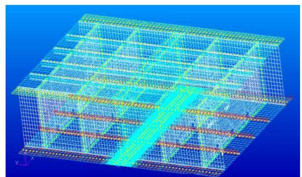
shows the whole finite element mesh generation.
