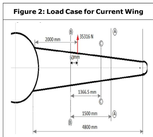
The load required at section C-C to stimulate the bending moment is  $P = 21361.57 \text{ N}$
