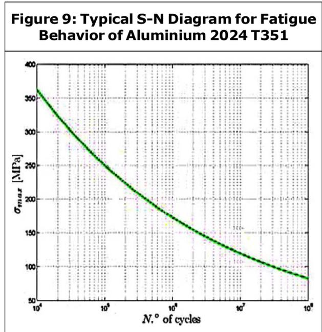
The simplest and most practical technique for predicting fatigue performance is the Palmgren-Miner hypothesis. The hypothesis contends that fatigue damage incurred at a given stress level is proportional to the number of cycles applied at that stress level divided by the total number of cycles required to cause failure at the same level. If the repeated loads are continued at the same level unit failure occurs, the cycles ratio will be equal to one.
