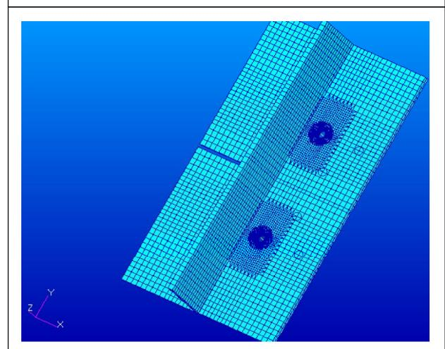
Average Stress value at a distance 85 mm to 90 mm from the spar tip is taken where maximum stress is identified in global analysis for calculation of load in local analysis and which is found to be 8.5 N/mm<sup>2</sup>.
