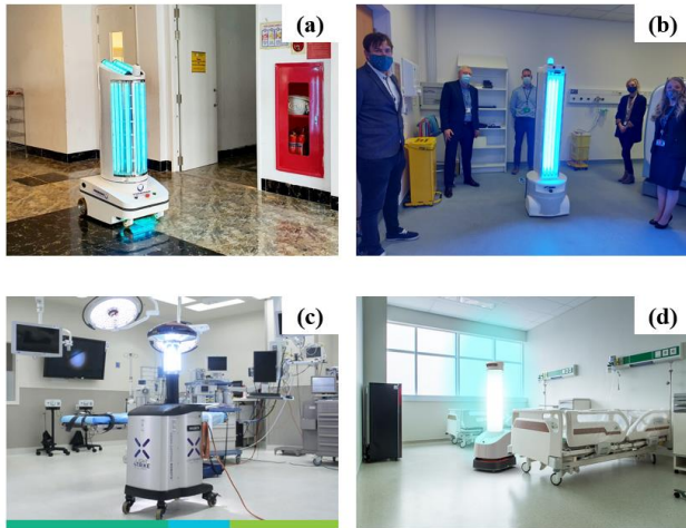
Figure 2. Photos of UV-C robots: (a) Phenikaa – X, (b) Akara, (c) Xenex, and (d) UVD Robots (Source: Official websites).
