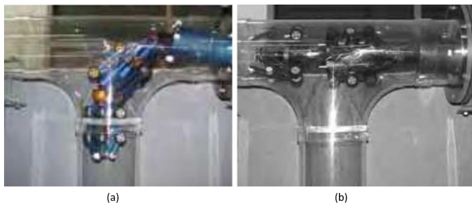
Figure 14. Active joint steering of robot in branch [64], (a) Steering inside T-branch, (b) Moves straightly inside T-branch without steering.
