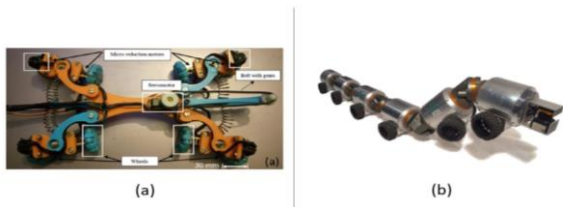
Figure 9. Prototypes of Bio-Inspired wheeled type IPIR. (a) Inspired by Spiders [61], (b) Inspired by Inchworms and Snakes [62].
