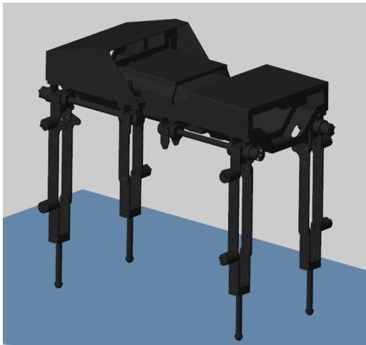
Figure 3. Quadrupedal robot model in simulation environment
