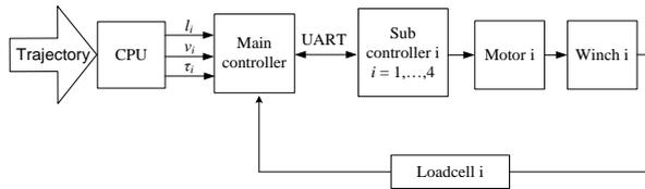
Figure 5. Diagram of cable robot control system
