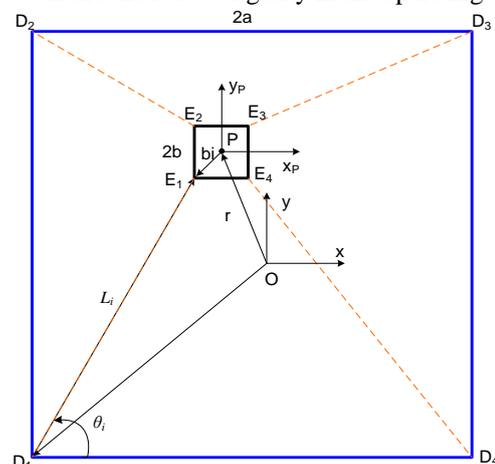
Figure 1. Kinematic structure of Planar CDPR
