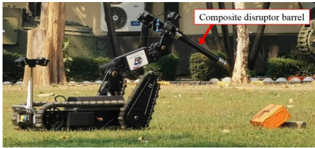
Figure 1. Composite disruptor barrel installed on DYNA-T
