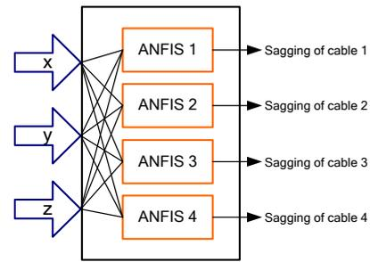
Figure 4. Proposed ANFIS architecture for cable sagging prediction
