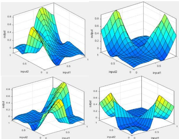
Figure 6. Response surface of ANFIS prediction system
