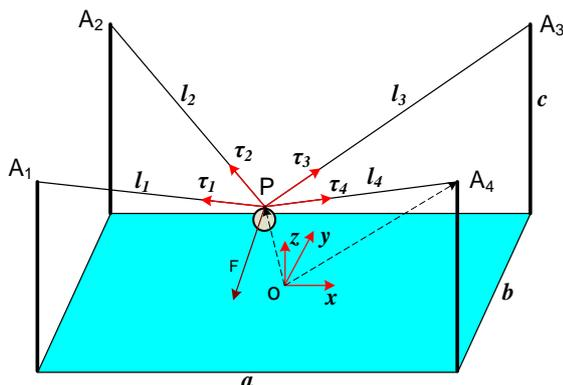
Figure 1. Cable robots with 4 sagging cables
