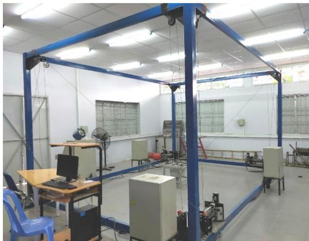
Figure 11. Cable robotic system in experiments.
