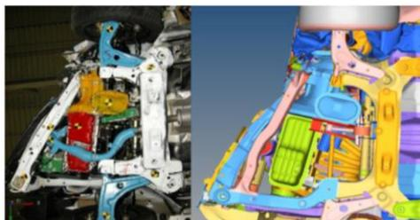
Figure 9. Comparison of frontal impact tests with analytical vehicular tests
