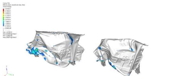
Figure 16. Trunk 30 km/h Deformation SPOT-CO<sub>2</sub>
