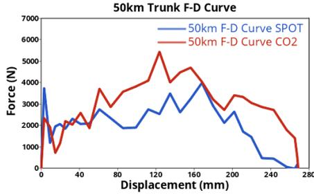
Figure 14. Trunk 50 km/h F-D Curve
