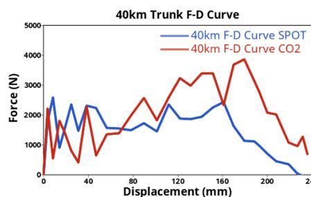
Figure 13. Trunk 40 km/h F-D Curve
