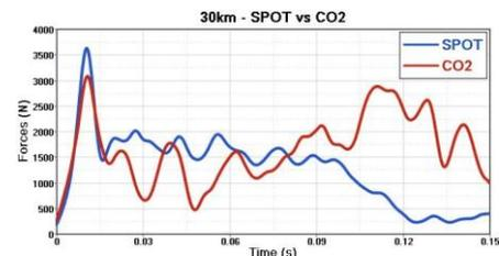
Figure 20. Trunk 30 km/h Force SPOT-CO<sub>2</sub>
