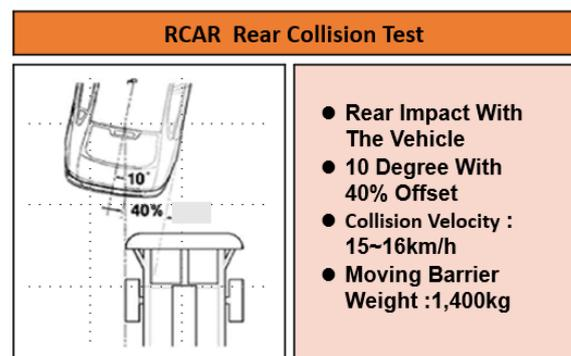
Figure 1. RCAR Rear Collision test
