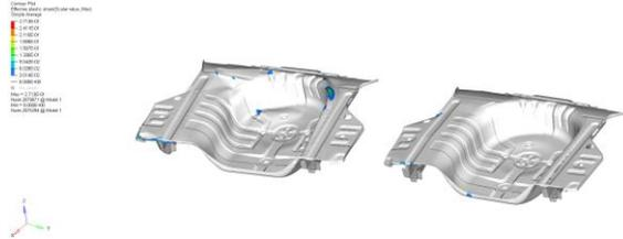
Figure 15. Trunk 15 km/h Deformation SPOT-CO<sub>2</sub>
