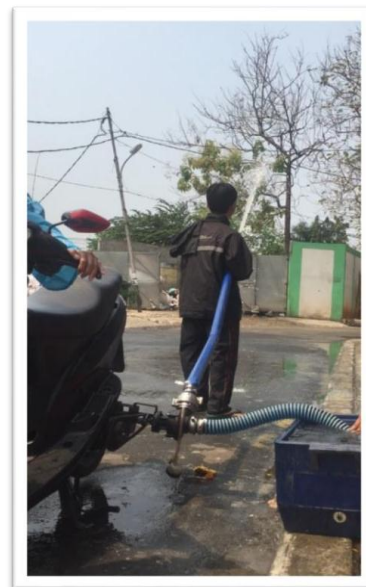
Figure 10. The nozzle testing on a centrifugal pump for a firefighting motorcycle.
