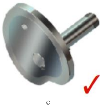
Figure 1. Drilling machine Dürselen PB.04N (a), and its cardioid cam (b,c)
