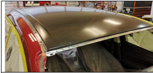
Figure 6. A vehicle with a new roof installed.
