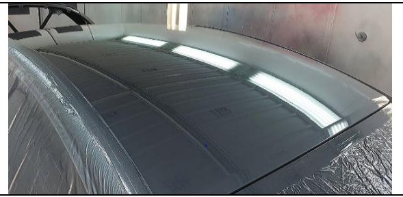
Figure 7. Painting operation following the roof repair.
