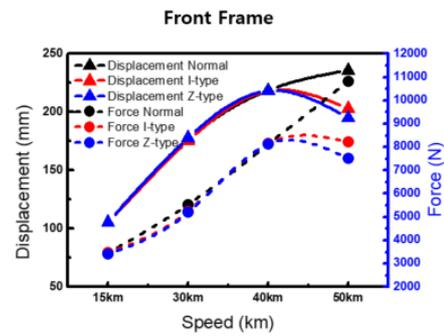
Figure 7. Speed of the front frame/deformation volume
