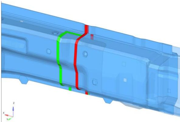
Figure 12. Type of Front Framework Weld I or Z
