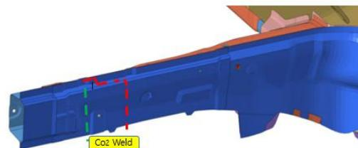
Figure 3. Front frame structure and post repair weld geometry
