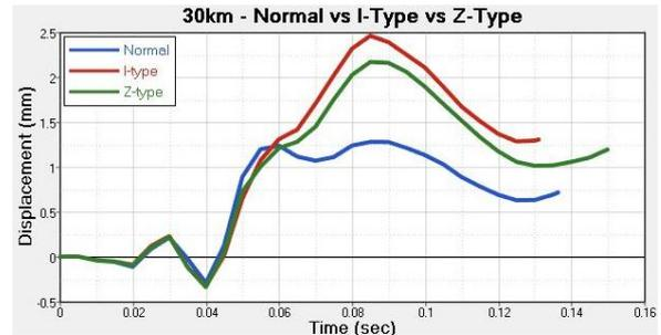
Figure 14. Front frame at 30km/h Displacement
