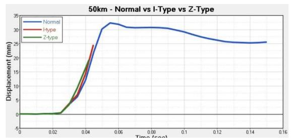
Figure 16. Front frame at 50km/h Displacement
