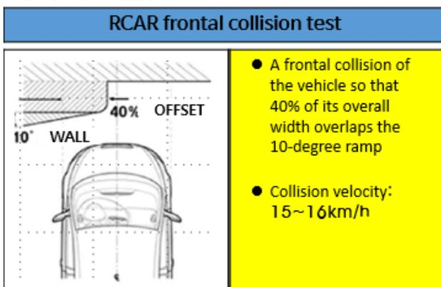
Figure 1 . RCAR collision test model
