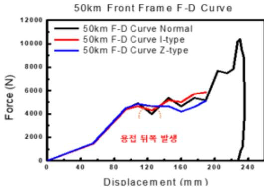
Figure 11. Front frame at 50km/h F-D Curve
