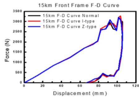
Figure 8. Front frame at 15km/h F-D Curve
