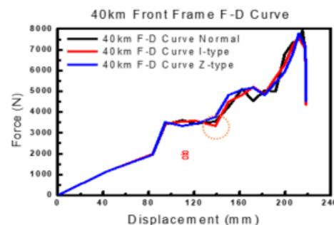
Figure 10. Front frame at 40km/h F-D Curve
