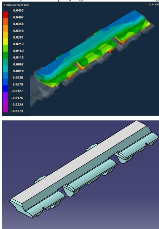
Figure 17. Chain piece made by sand casting, the Y displacement (cm) happens during the solidification process.
