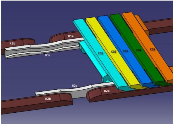
Figure 9. SimDesigner simplified model for rigid body collision analysis. The track is denoted by R1a, R1b, R2a, and R2b; R1c and R2c denote the guide slot; c-01 denotes the five chain pieces to c-05.
