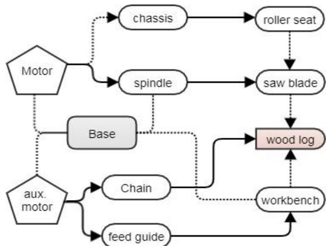
Figure 6. The relative functional components and their relation to the cutting marks.
