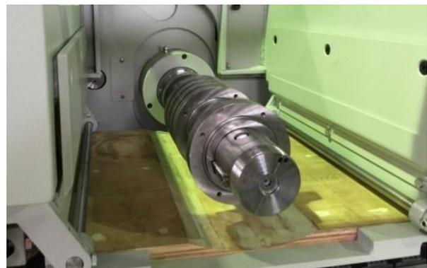
Figure 1. Multi-piece groove spindle.
