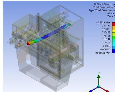
Figure 15. The deformation and stress distribution of the spindle are 0.36mm and 25M
