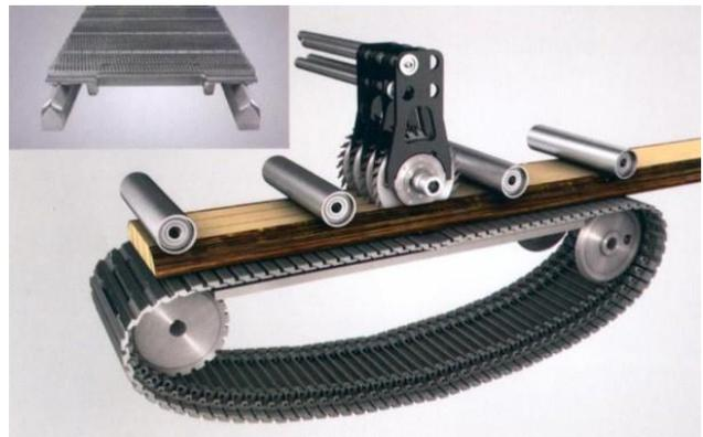
Figure 5. The internal chain, roller, and rip-saw of the woodworking machine (<https://www.oavequipment.com>)
