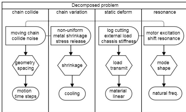
Figure 8. Related mechanical engineering principles of multiple engineering analysis
