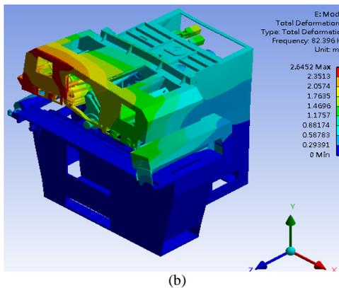
Figure 16. The mode-8 is resonant at the roller seat, in which the stand is twisted. The original machine (a) is 78.8Hz, and the modified design (b) is 82.3Hz [14]
