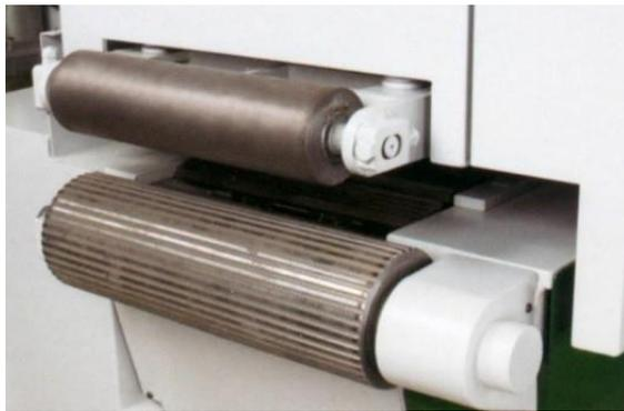
Figure 3. An auxiliary power wheel
