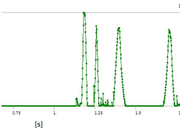
Figure 10. Rigid body impact force on c-02: Adding the guide groove (upper and lower clearances were 0.2 and 0.8 mm, respectively), the impact amplitude at the c-02 changed to be 1019 N.
