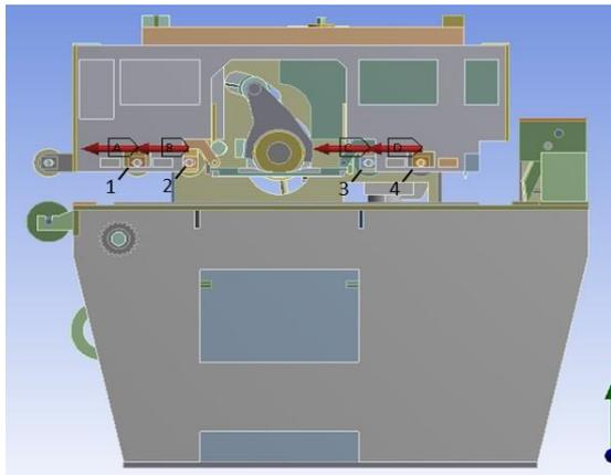
Figure 12. The roller shaft is subjected to the -X direction force placed on location A,B,C,D, and the displacement calculations of roller seats are placed on location 1,2,3,4.
