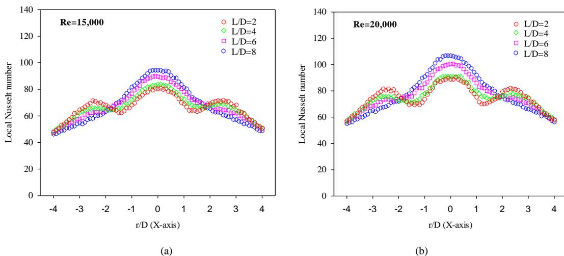
Figure 4. Effect of the nozzle-to-plate spacing ( $L/D$ ) on local Nusselt number distribution of the conventional impinging jet (CIJ).
