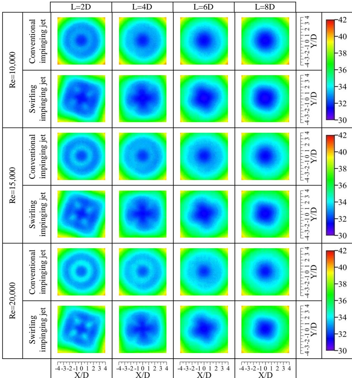
Figure 3. Temperature distribution on impinging plate.
