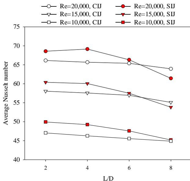
Figure 7. Effect of multi-channel twisted tape on average Nusselt numbers.
