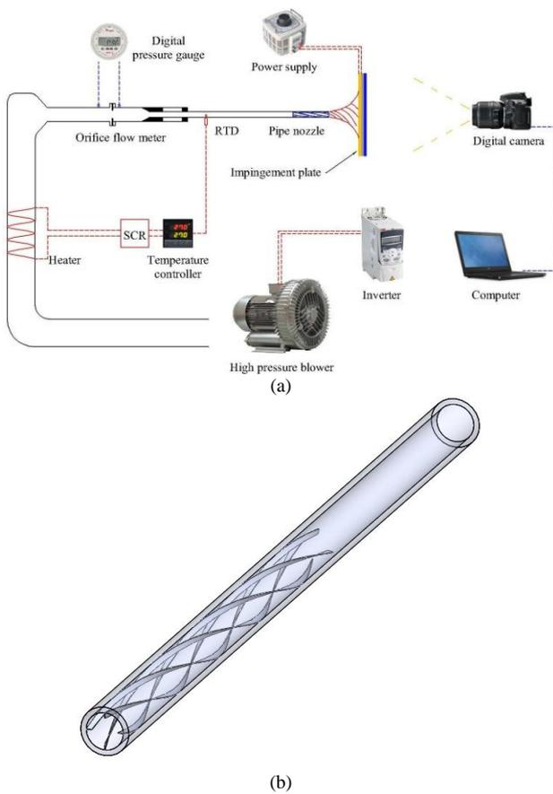
Figure 1. Layout of experimental facility and nozzle with centrally hollow twisted tape
