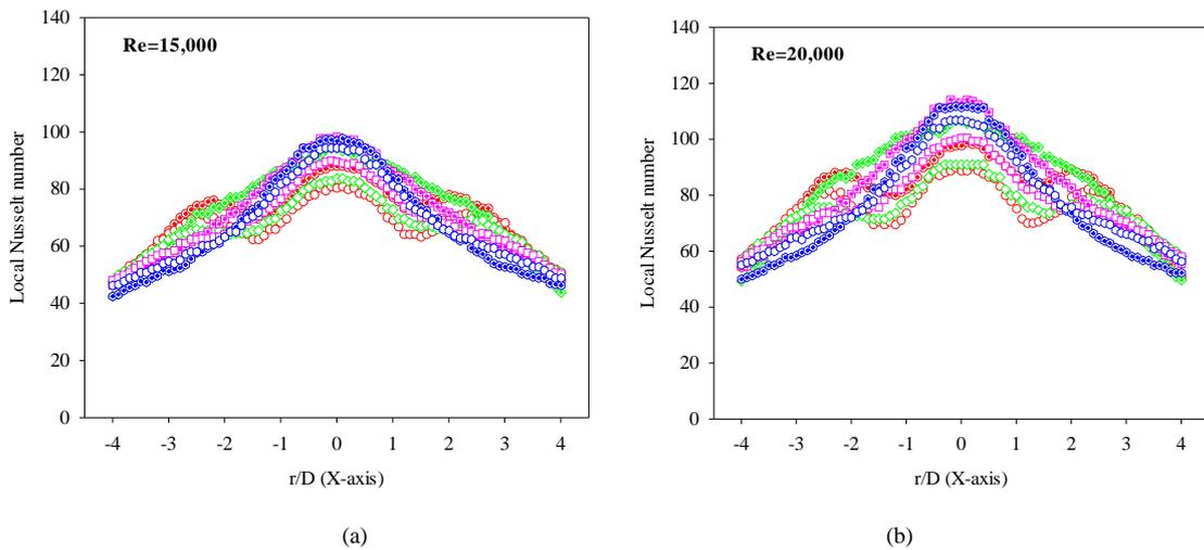
Figure 6. Effect of the nozzle-to-plate spacing ( $L/D$ ) on local Nusselt number distribution of the swirling impinging jet (SIJ)
