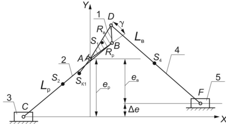
Figure 2. Kinematic chain of rhomboid mechanism of Stirling engine with forked crank: 1 – forked crank, 2 – working pin’s conrod, 3 – working pin, 4 – displacing pin’s conrod, 5 – displacing pin;  $S_1, S_2, S_3$  – mass centers of links with masses  $m_1, m_2, m_3$ ;  $R_d$  and  $R_w$  – cranks parts lengths for working and displacing groups,  $L_d$  и  $L_w$  – lengths of displacing and working conrods,  $e_d$  и  $e_w$  – eccentricity of pins,  $\gamma$  – crank angle
