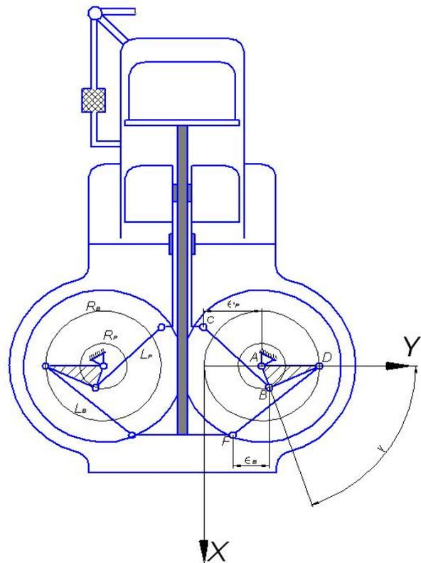
Figure 1. Generalized scheme of Stirling engine with forked crank.
