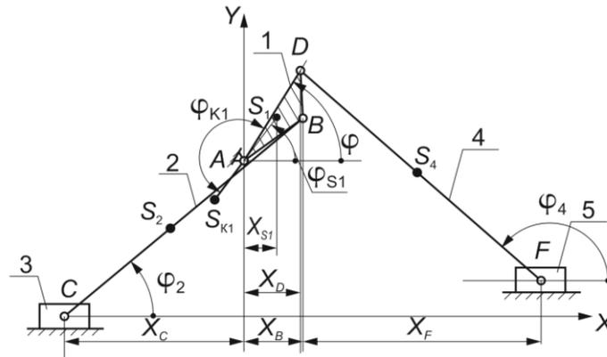
Figure 3. Calculation scheme for pointed masses
