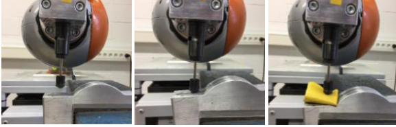
Figure 2 Normal clamping position (left); Altered clamping position (middle); Disturbance through intruding material (right).
