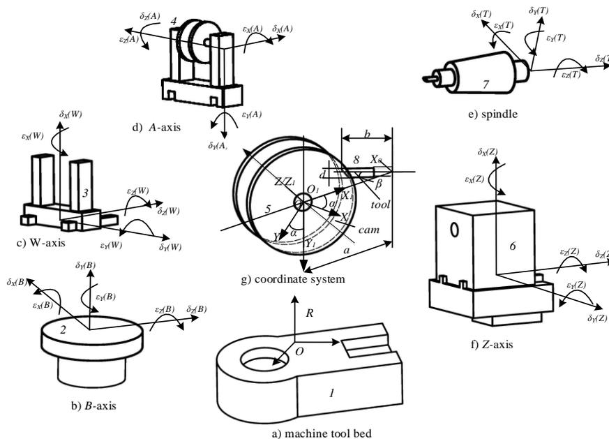
Figure 2. Error definition of special machine tool.
