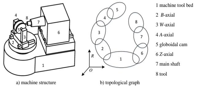
Figure 1. Topology diagram of special machine tool.
