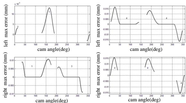
Figure 5. Profile error variation curve of maximum groove depth at  $\Delta\alpha=0.01^\circ$ .
