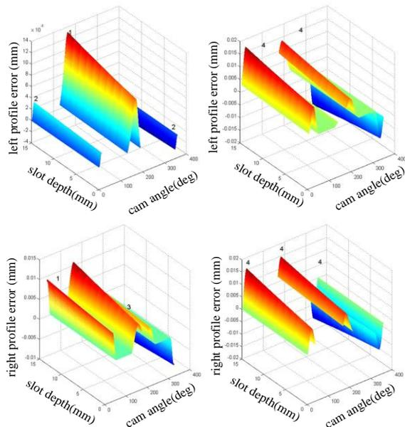
Figure 4. Profile error at  $\Delta\alpha=0.01^\circ$ .
