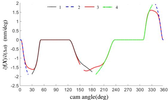
Figure 3. Influence coefficient curve of cam rotation error  $\Delta\alpha$ .
