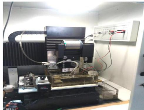
Plate 1 Micro WEDM of Al7075 work piece on DT 110 micro machine
