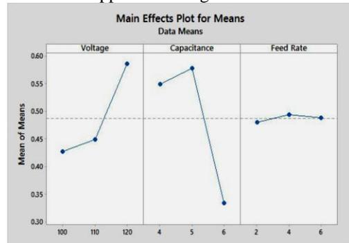
Figure 4. Main Effect Plot for means of Grey Relational Grade
