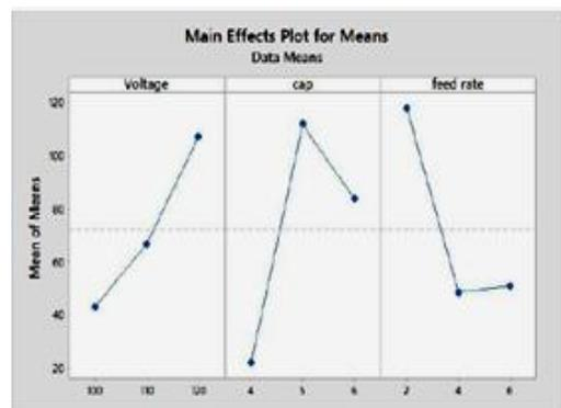
Figure 2. Main effects Plot for the means of MRR.
