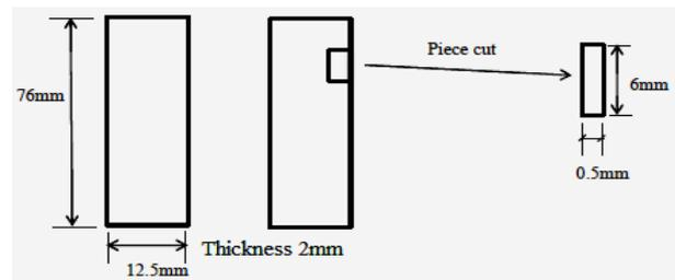
Figure 1. Machined work piece dimensions and schematics
