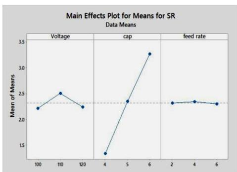
Figure 3. Main Effects Plot for the means of Surface Roughness
