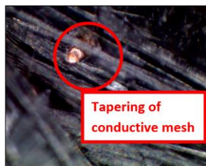
Figure 7. Tapering of the conductive mesh.
