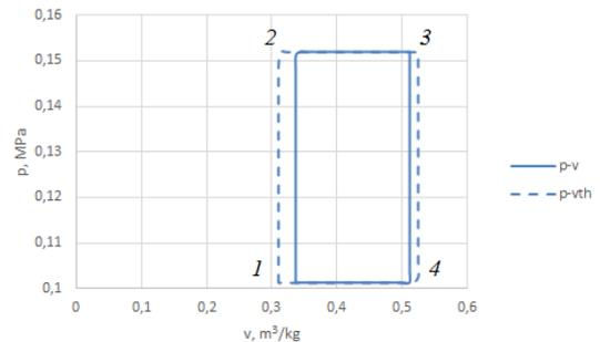
Figure 6. p-v diagram for thermocompressor.
