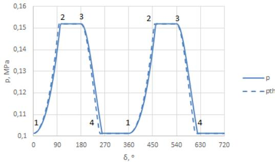
Figure 7. Pressure change in thermocompressor.
