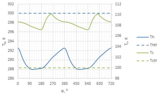
Figure 3. Distribution of the gas temperature in hot and cold chambers.
