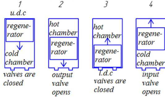
Figure 2. Working cycle of the thermocompressor.
