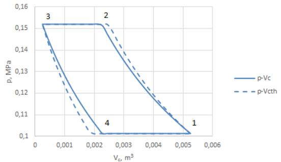
Figure 5. p-v diagram for cold chamber.
