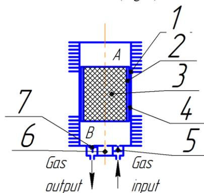
Figure 1. Principal scheme of the mechanical thermocompressor:
