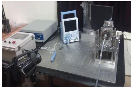
Figure 6. Test using hybrid NDT system
