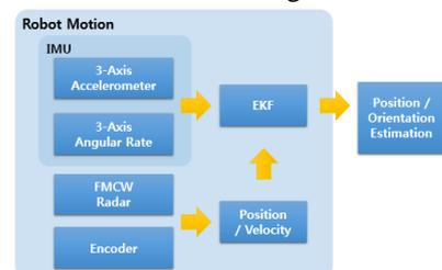
Figure 2. Configuration of the system
