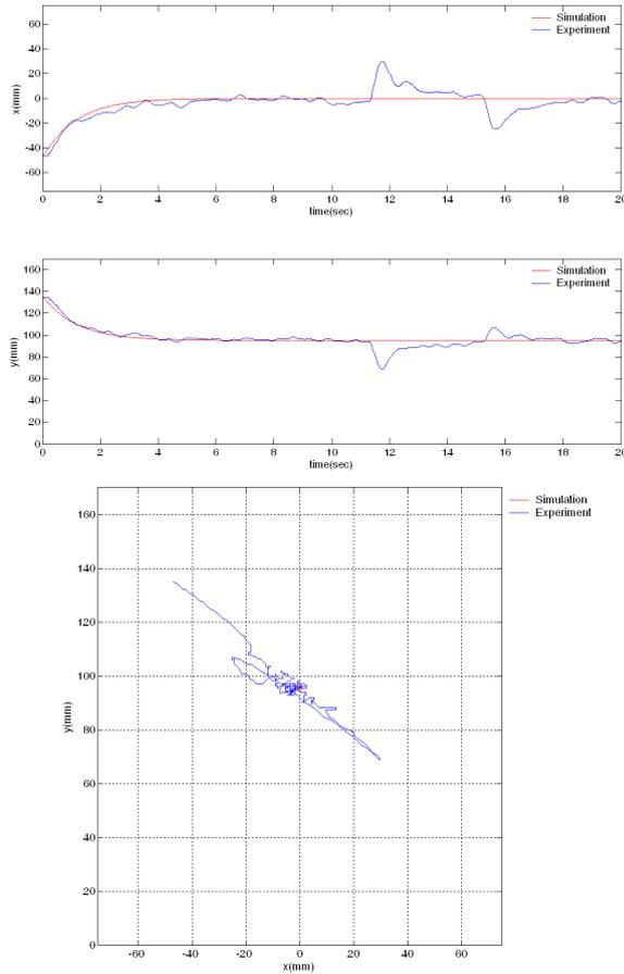
Figure 5. Position responses and planar trajectory of the balancing experiment.
