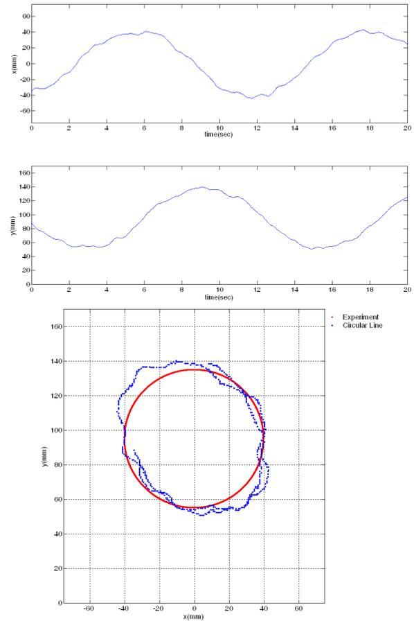
Figure 6. Position performance along  $x$  and  $y$  directions and planar trajectory for tracking a circular path.
