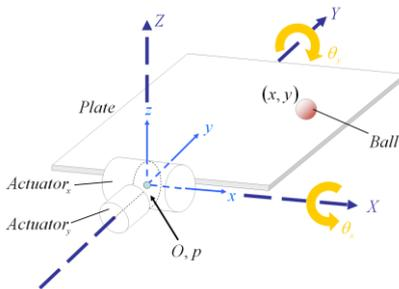
Figure 2. Coordinate systems for the ball-plate system.
