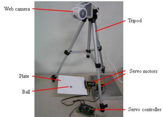
Figure 4. The experimental setup for balancing the ball-plate system.
