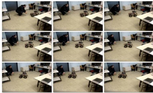
Figure 11. Robot detecting human obstacle and reducing speed.
