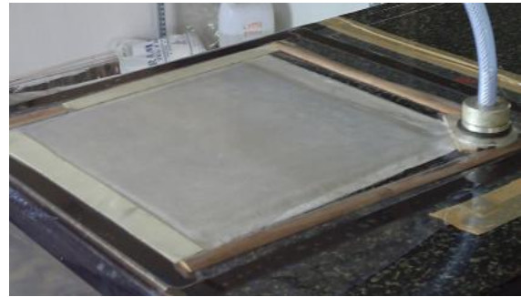
Figure 2: Vacuum Bag Process
