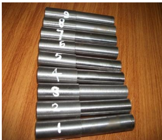
Figure 3: EN-8 Steel Rods (After Turning)
