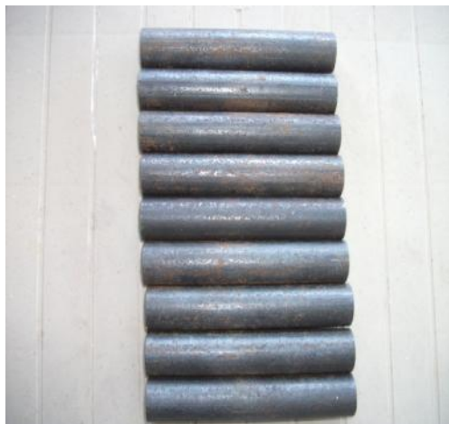
Figure 3: EN-8 Steel Rods (After Turning)
