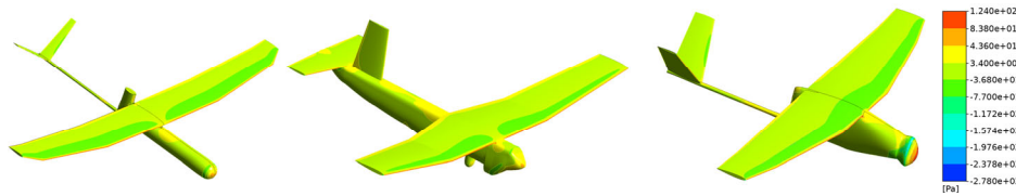
Fig. 5. Surface pressure contours of UAV 1, UAV 5, and UAV 7 with a common pressure legend (Cruise speed: 14 m/s).
