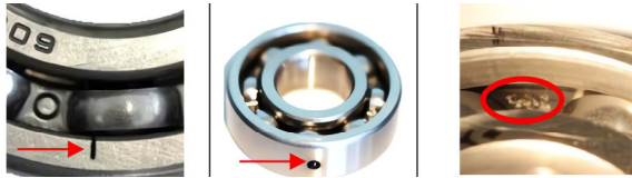
Fig. 3. Artificial bearing damage patterns documented in the Paderborn dataset [48]. Controlled defects include drilled holes and engraved cracks at predetermined locations.
