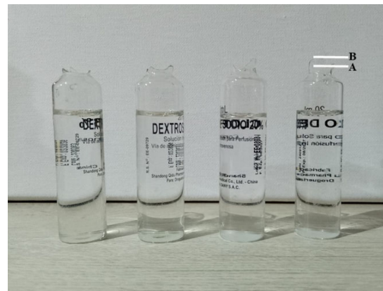
Fig. 10. Length of the sharp edge of the ampoules opened by the ampoule-breaking machine.
