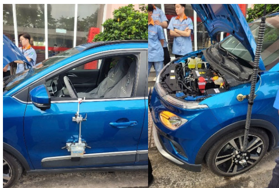
Fig. 6. Sensor layout for real-time vehicle braking data acquisition.
