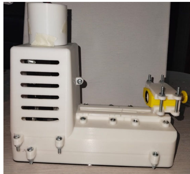
Fig. 7. Assembly of a drug reconstitution machine.
