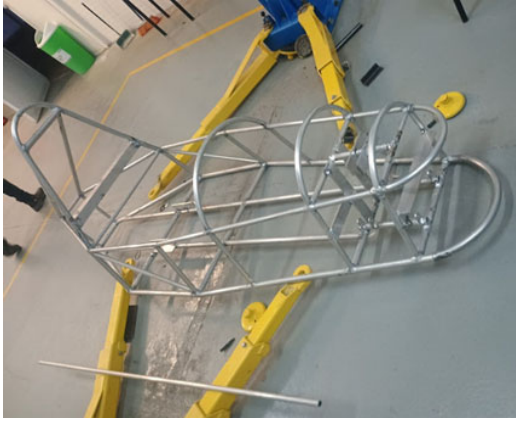
Fig. 28. Aluminum structure of the single seater completed.
