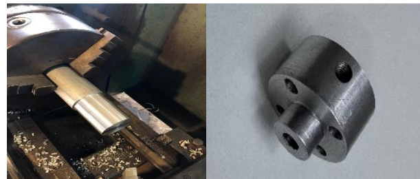
Fig. 3. Flange coupling Aluminium alloy.
