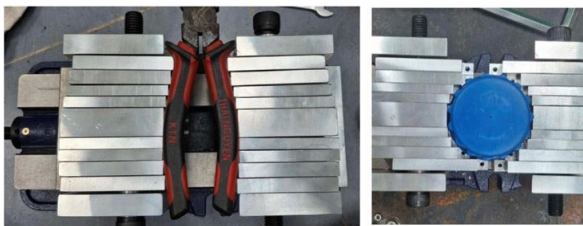
Fig. 10. Clamp testing on complex-contour parts: (left) asymmetric hand tools; (right) circular ribbed plastic component.
