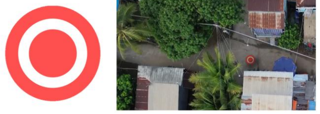
Fig. 4. The designed landmark on the left and its real-world counterpart on the right.
