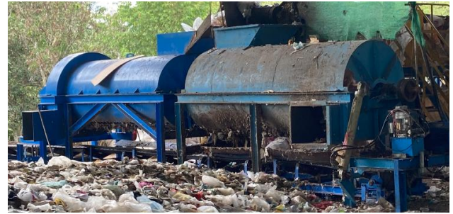
Fig. 12. The development plastic cleaning machine [Left] and the conventional plastic cleaning machine [Right] at landfill.
