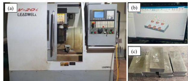
Fig. 1. LEADWELL V20i VMC (a) milling machine, (b) cutting simulation, and (c) workpieces.
