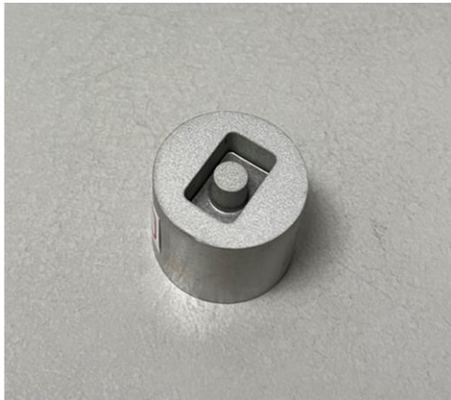
Fig. 6. Physical appearance of the rectangular groove with inner cylinder.
