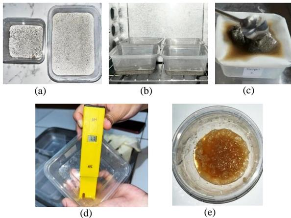
Fig. 2. Silica extraction process. (a) Drying the rice husk ash for 15 hours under the sun; (b) Dissolving rice husk ash with KOH and heated using an oven; (c) Filtering process to produce filtrate; (d) Addition of HCL to neutral pH; (e) Results of silica extract.
