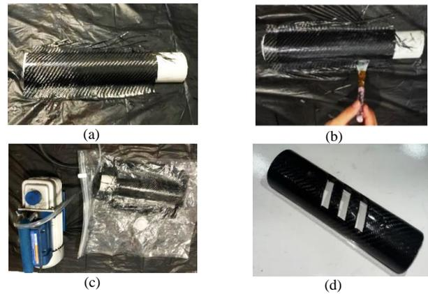
Fig. 3. CFRP manufacturing process. (a) Laying the carbon fiber on the surface that has been smeared with the matrix; (b) Layering of 5-times matrix and carbon fiber coatings; (c) Vacuum process; (d) CFRP composites.
