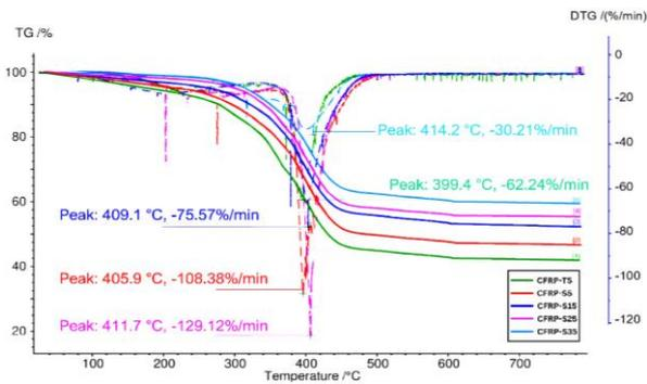
Fig. 9. Decomposition temperature curve.
