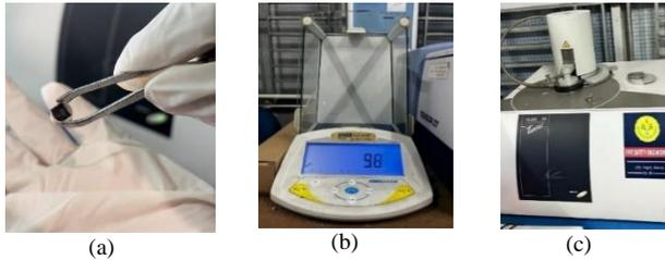
Fig. 4. Thermal stability testing process (a) Sample to be tested (b) Weighing the mass of the sample before testing (c) Sample testing process with TGA machine.
