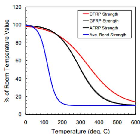
Fig. 1. Properties of FRP (Carbon, Glass, and Aramid) at elevated temperatures.
