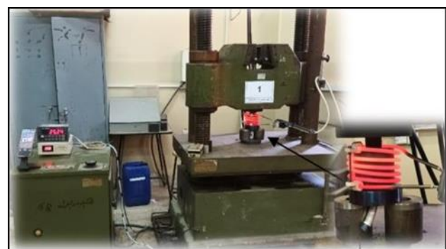
Fig. 3. The SANS 100Ton hydraulic press is used in the extrusion process, its accessories, and the method of heating the die.
