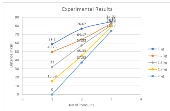
Fig. 13. Carrying capacity trend in pushing mission under 5 varying loads.
