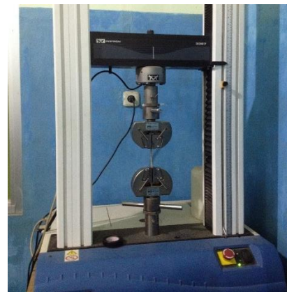
Fig. 2. PP and corn stalk specimen. (a) Specimen dimension of ASTM D 638-04. (b) Specimens after cutting process. (c) Samples for SEM and water absorption. (d) The sample attached to the UTM.
