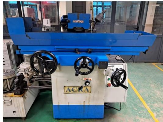
Fig. 1. Surface Grinding Machine APSG-820/2A
