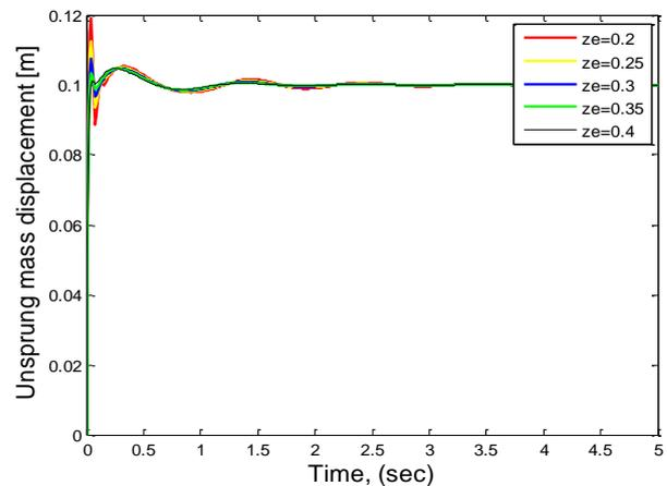
Fig. 5. Unsprung mass displacement for damping ratio 0.2 to 0.4
