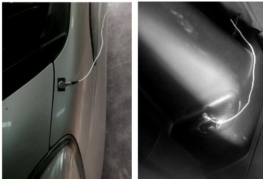
Fig. 11. Location of accelerometer.
