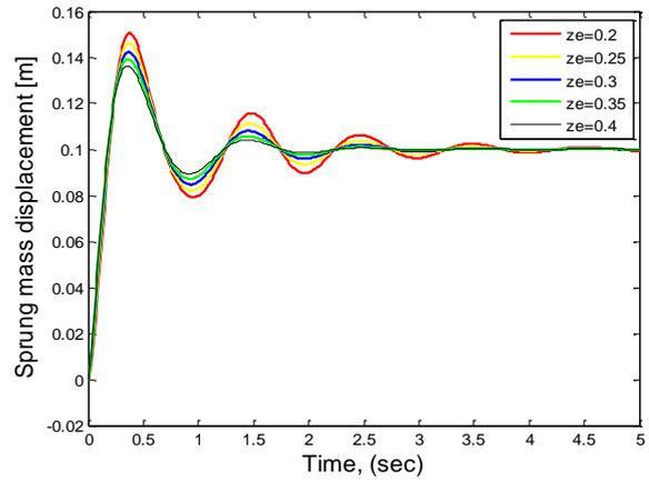
Fig. 4. Sprung mass displacement for damping ratio 0.2–0.4.
