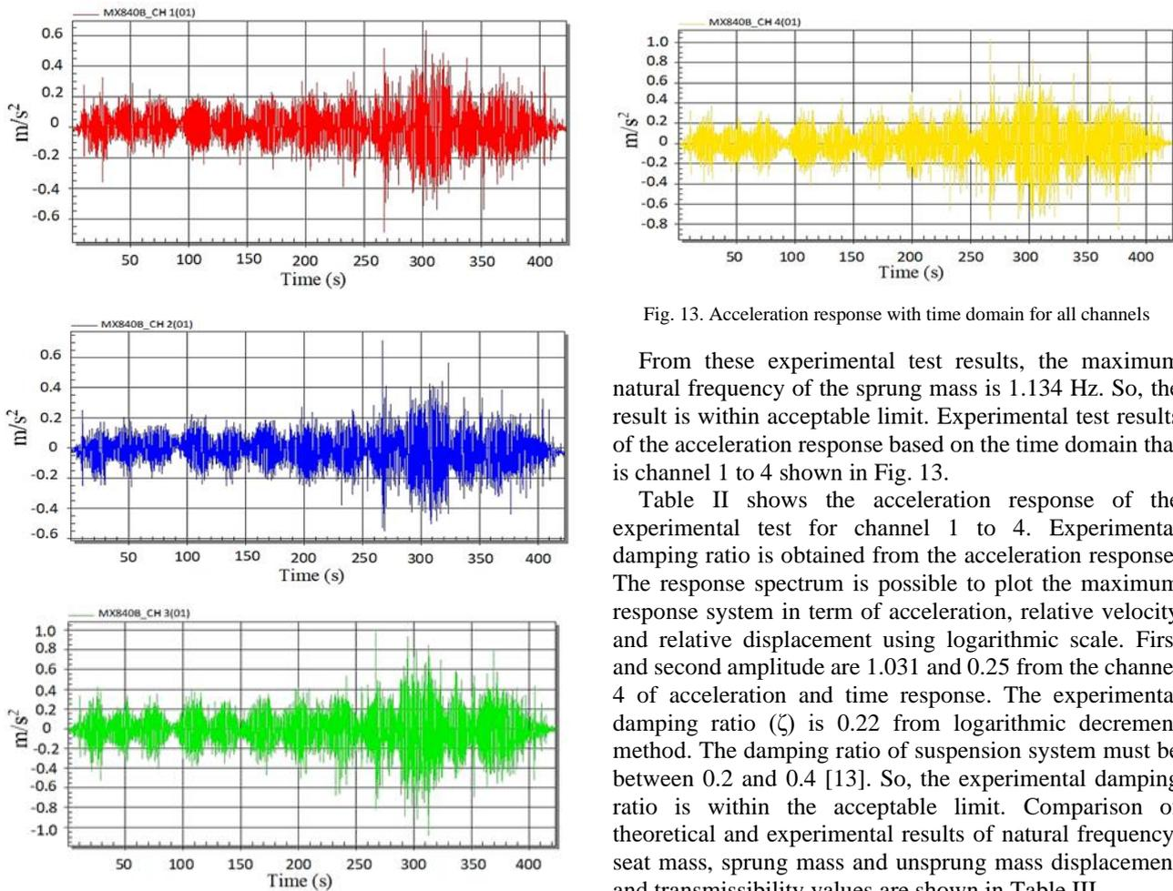
Fig. 13. Acceleration response with time domain for all channels
