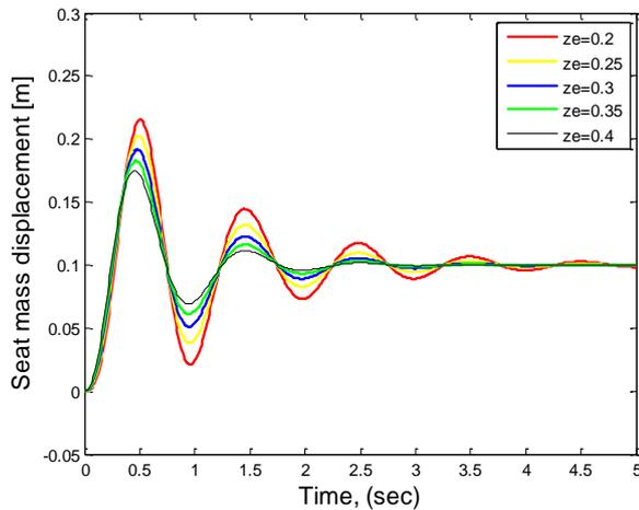
Fig. 3. Seat mass displacement by changing damping ratio 0.2–0.4.
