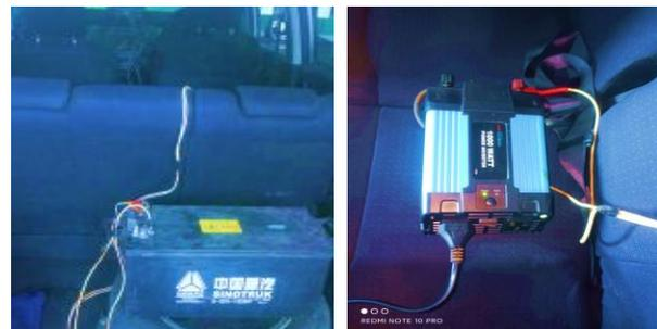
Fig. 9. 12V battery and AC to DC converter.
