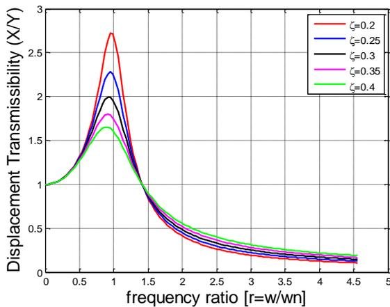
Fig. 7. Displacement transmissibility for damping ratio 0.2 to 0.4.
