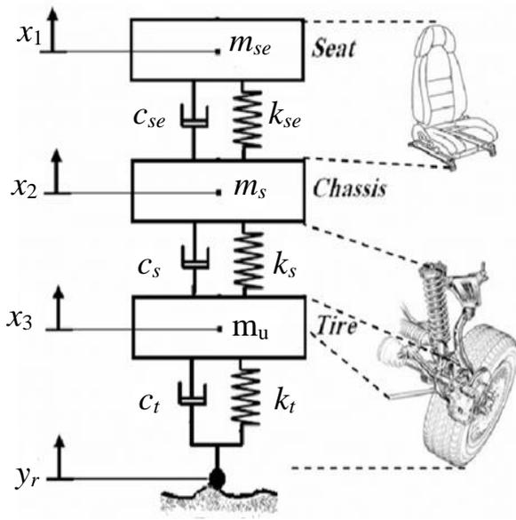
Fig. 1. 3DOF quarter car model with tire damping [15].
