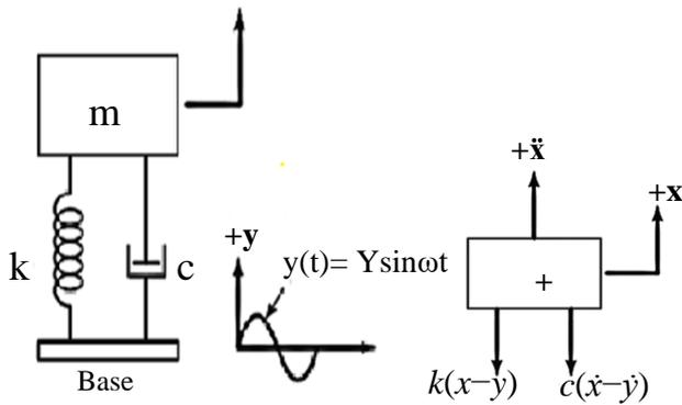
Fig. 6. Base excitation model and free body diagram [13].
