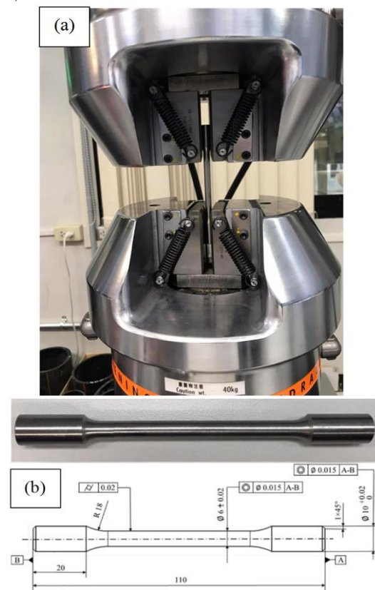
Fig. 2. Tension testing equipment including (a) The tensile testing machine (b) The geometry of the standard specimen (all dimensions are in millimeter).
