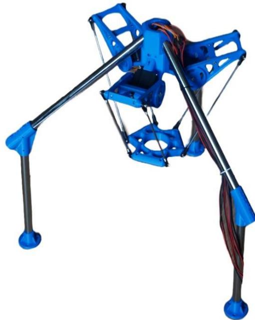
Fig. 3. Assembled delta robot.
