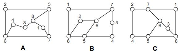
Figure 3. Three eight bars kinematic configurations, such as B and C isomorph and A non-isomorph with B and C.
