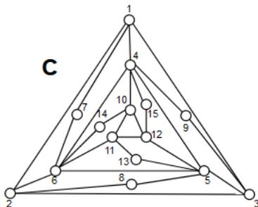
Figure 6. fifteen bars kinematic chains configurations isomorphic with Fig. 4.
