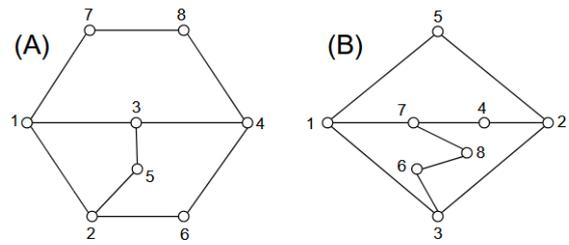
Figure 12. Two isomorphic eight bars kinematic chains
