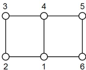
Figure 10. Wall graph kinematic chain.
