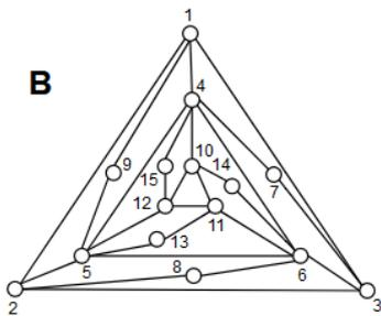
Figure 5. fifteen bars kinematic chains configurations non-isomorphic with Fig. 4.
