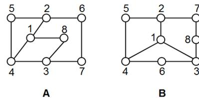
Figure 11. Two non-isomorphic eight bars configuration
