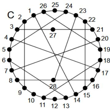
Figure 9. Twenty-eight bars kinematic chains non-isomorphic with Fig. 7.
