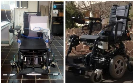
Figure 1. Autonomous wheelchair prototype.
