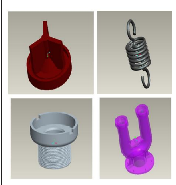
Figure 2: Parts of Spring Operated Relief Valve
